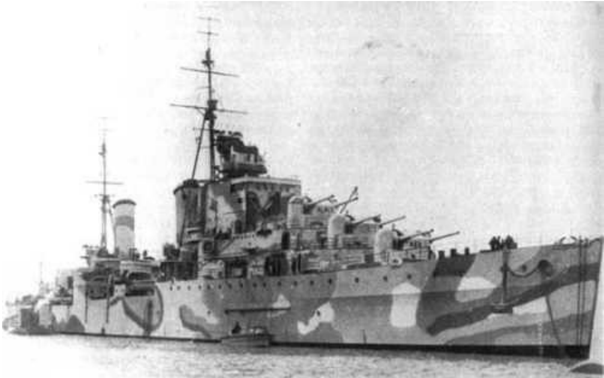
HMS CLEOPATRA – radar Type 960 and 5.25 Turrets in A, B and C turrets, so probably taken about Terence's time
