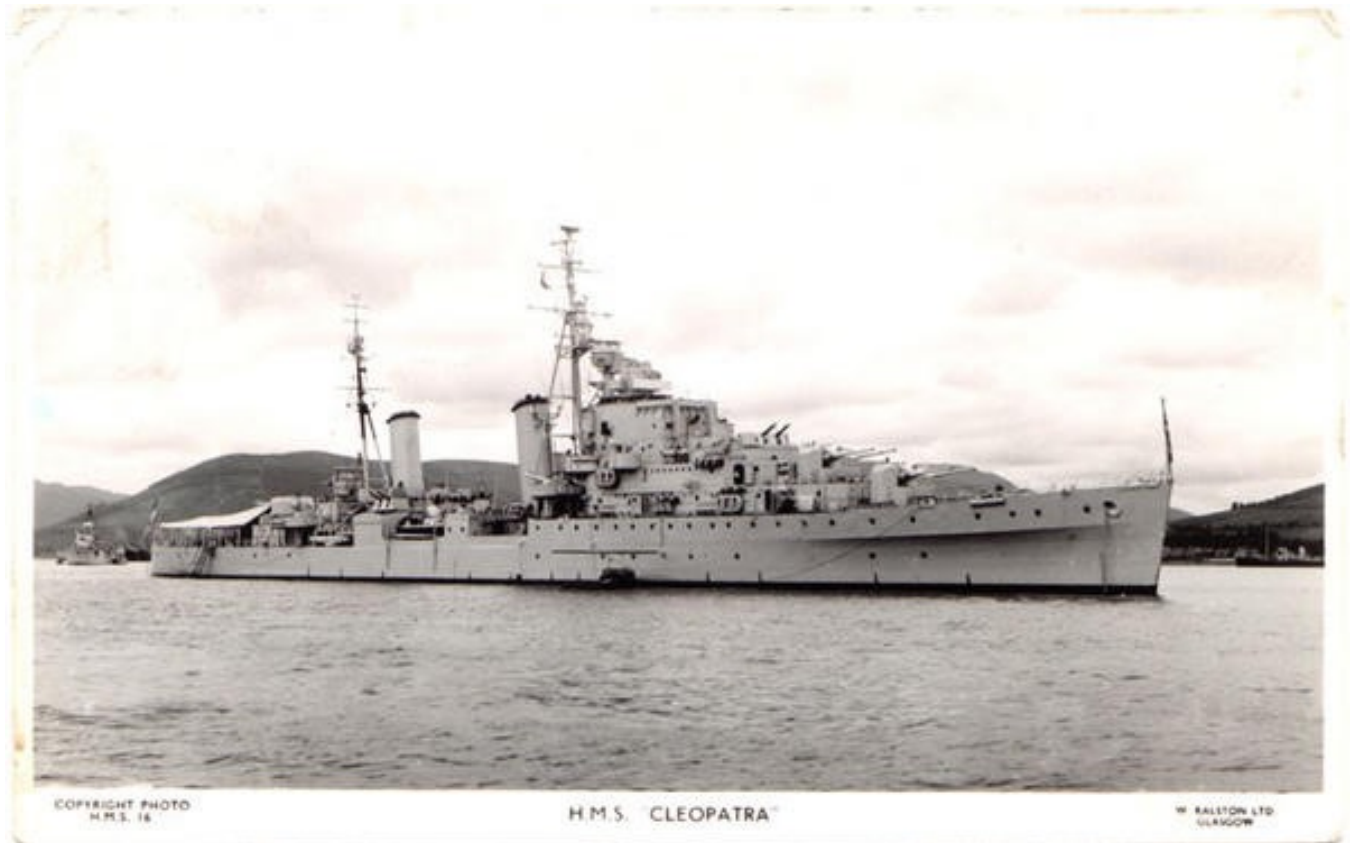
HMS CLEOPATRA . Photograph probably post WW2, Radar Type 293 and a different calibre gun in C Turret
